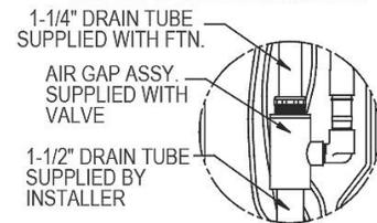
**SANITARY FREEZE-RESISTANT VALVE GROUND INSTALL DETAIL**
