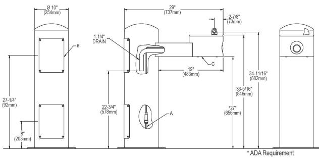
A = 3/8" O.D. Unplated copper tube connect shut off valve by others B = Access Panel (8" X 10") C = Removable bottom cover
