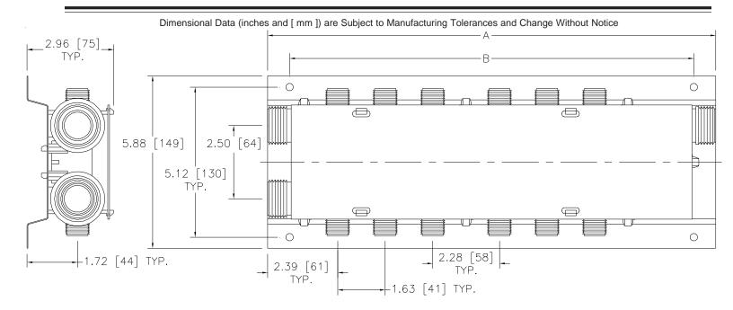
Engineering Specification: ZurnPEX® 1" diameter polysulfone QickPort® Preassembled Manifold. Comprised of hot and cold 1/2" male straight pipe thread outlets and 1" male straight pipe thread inlets. Manifold is rated at a maximum pressure of 100 PSI at 180°F. Optional shut off valves can be added for individual on/off control of each distribution line. NSF listed. For use with potable water only.
