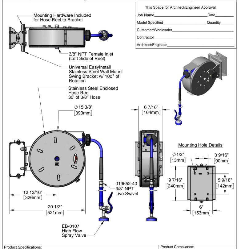
3/8" x 30' Stainless Steel Enclosed Reel, High Flow Spray Valve w/ swivel &
