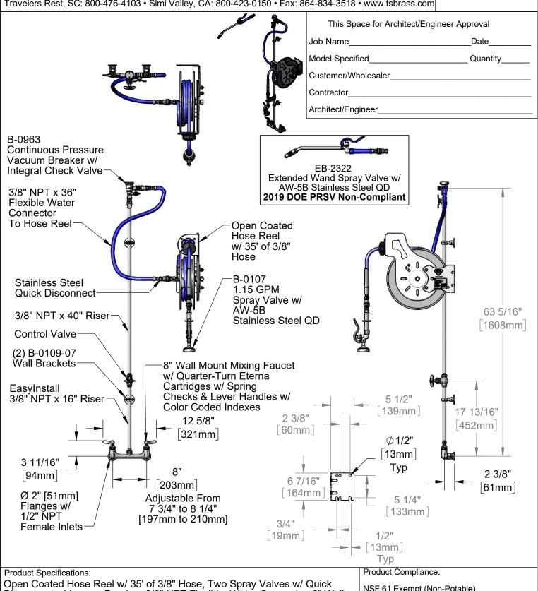
Open Coated Hose Reel w/ 35' of 3/8" Hose, Two Spray Valves w/ Quick Disconnects, Vacuum Breaker, 3/8" NPT Flexible Water Connector, 8" Wall Mount Mixing Faucet & Control Valve
