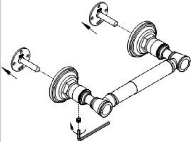
② ALIGN MOUNTING BRACKETS AND MARK LOCATION
