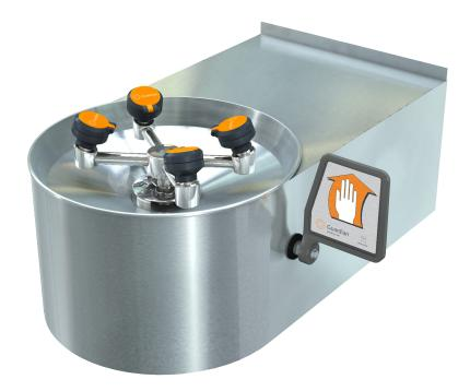
**Application:** Barrier-Free WideArea<sup>™</sup> eye/face wash for wall mounting. Bowl is lowered and extended to permit access by wheelchair user. Profile of unit is "flattened" to comply with maximum height and knee clearance requirements. Unit has stainless steel bowl and wrap-around skirt to conceal valve, drain and piping.
